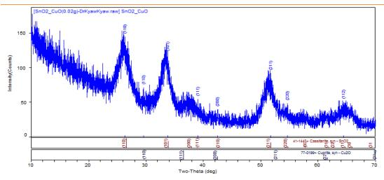
Fig 3(a). XRD profiles of SnO<sub>2</sub>:CuO (0.02g) thin film.
