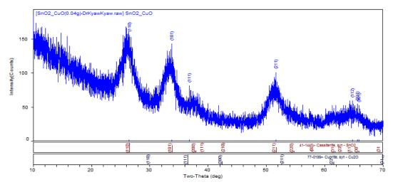
Fig 3(b). XRD profiles of SnO<sub>2</sub>:CuO (0.04g) thin film.
