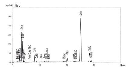
Fig 2. The amount of count versus energy spectrum of the SnO<sub>2</sub>:CuO thin film.
