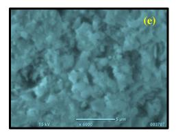
Fig 4. The SEM micrographs of SnO<sub>2</sub>: CuO nanostructured thin films.
