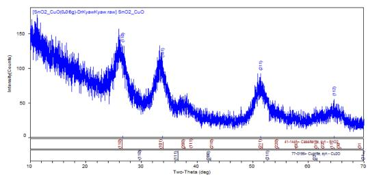
Fig 3(d). XRD profiles of SnO<sub>2</sub>:CuO (0.08g) thin film.
