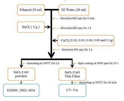
Fig 1. The block diagram for the fabrication of SnO<sub>2</sub>: CuO nanostructured thin films.
